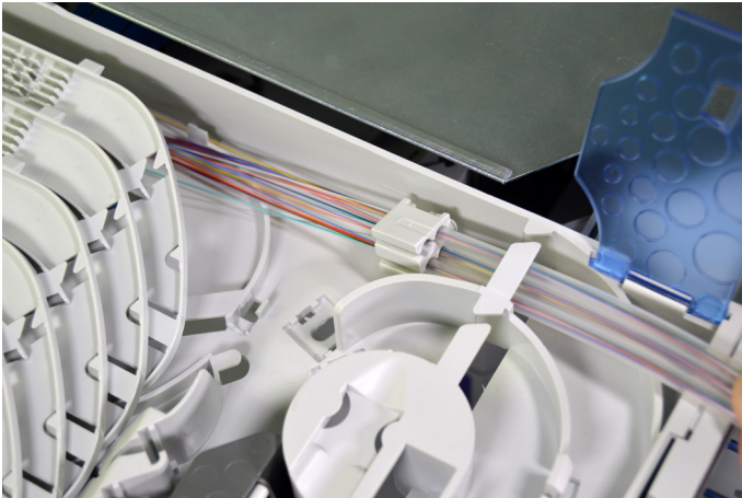
6.1.9. Slide the other sides of the transportation tubes in the other tube holder. Open the lids. Push / slide all transportation tubes one by one into the tray.
