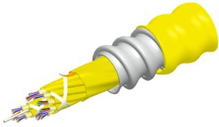
Fiber indoor cable, TeraSPEED® Riser/LSZH rated, MPO Trunk, interlocking aluminum armored, Singlemode G.652.D and G.657.A1, 24 fiber with 12 fiber subunits, Feet jacket marking, Yellow jacket color
