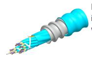
Fiber indoor cable, LazrSPEED® Riser/LSZH rated, MPO Trunk, interlocking aluminum armored, Multimode OM4, 144 fiber multi-unit with 12 fiber subunits, Gel-free, Feet jacket marking, Agua jacket color
