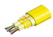
Fiber indoor cable, TeraSPEED® Low Smoke Zero Halogen Riser MPO Trunk, 32 fiber with 16-fiber with 3.0 mm subunits, Singlemode G.657.A2 /B2, Feet jacket marking, Yellow jacket color, B2ca flame rating
