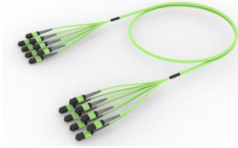
Ultra Low Loss (ULL) OM5 MPO8 (Non-Pinned) to MPO8 (Pinned), Fiber Trunk Cable Assembly, 64-Fiber, Dual Rated (OFNR/LSZH)
