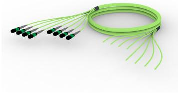
Ultra Low Loss (ULL) OM5 MPO APC (Non-Pinned) to Unconnectorized, Fiber Trunk Cable Assembly, 64-Fiber, Dual Rated (OFNR/LSZH)
