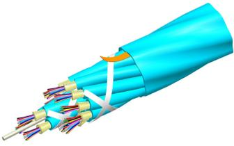
Fiber indoor cable, LazrSPEED® Low Smoke Zero Halogen Riser MPO Trunk, 64 fiber multi-unit with 8 fiber 2.0mm subunits, Gel-free, Multimode OM5, Feet jacket marking, Aqua jacket color, Dca flame rating
