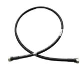
HELIAX® 1/2" Superflexible Fire retardant SureFlex® Jumper with interface types 4.3-10 Male and 4.3-10 Male, 2m, with black non-halogenated fire retardant polyolefin jacket
