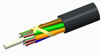
Fiber OSP cable, LightScope® ZWP Blown Micro Single Jacket, 36 fiber, All-Dielectric Stranded Loose Tube Arid-Core™ Construction, Gel-filled, Singlemode G.652.D and G.657.A1, Feet jacket marking, Black jacket color
