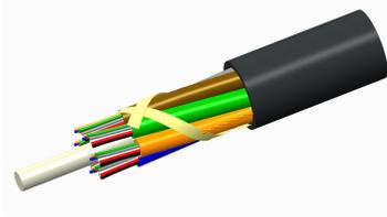
Fiber OSP cable, LightScope® ZWP Blown Micro Single Jacket All-Dielectric Outdoor Stranded Loose Tube Arid-Core™ Construction, 144 fiber, Singlemode G.657.A1, Gel-filled, Meters jacket marking, Black jacket color
