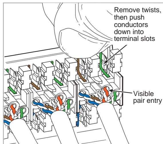
Figure 5. Seat Untwisted Pairs into IDC Terminal Slots
