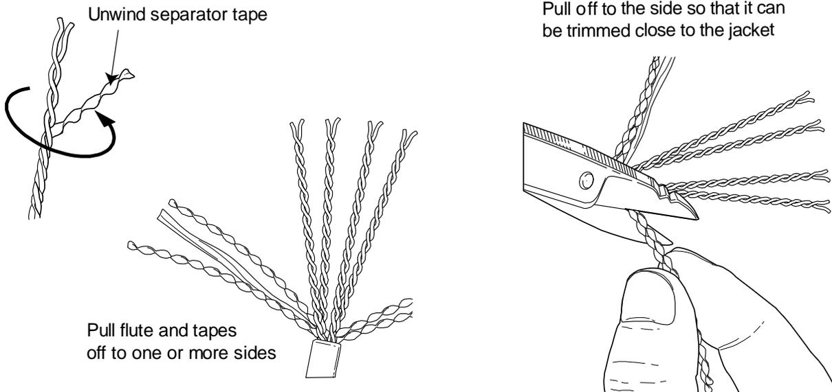
Preparation of the **SYSTIMAX GigaSPEED X10D 91B series cable, 95B series cordage, or Xpress® 88 series cable** is shown above. For complete instructions on preparing the **GigaSPEED X10D 91B series cable, 95B series cordage, or Xpress® 88 series cable** for termination, see instruction sheet 860469402.
