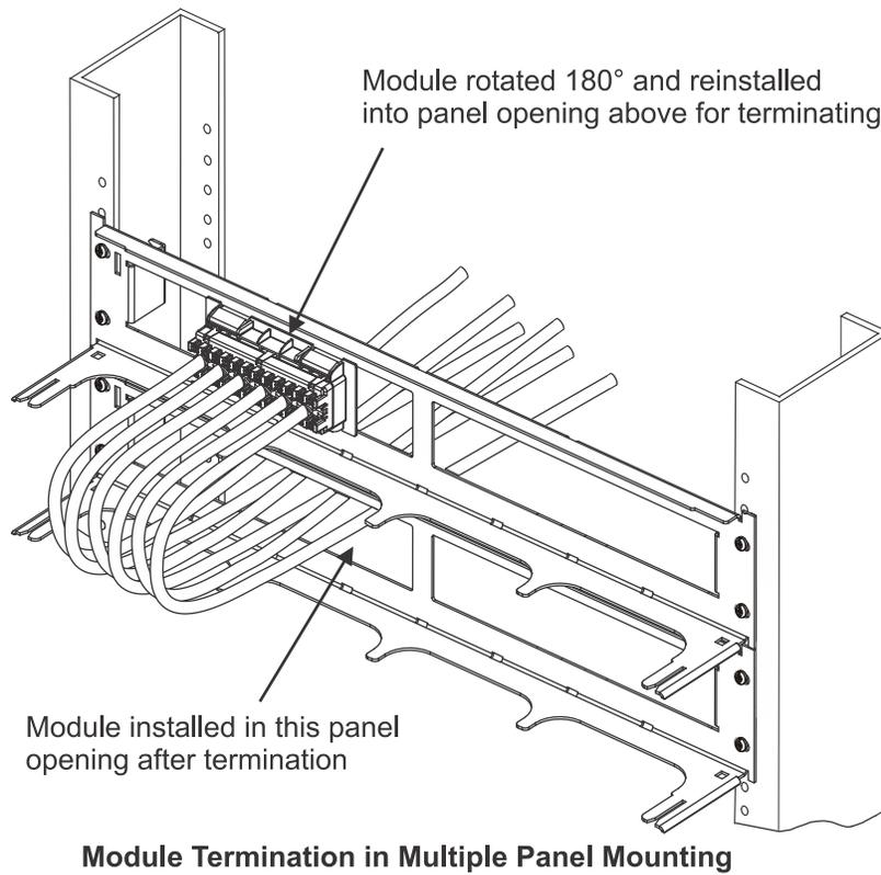
**Module Termination in Multiple Panel Mounting**
