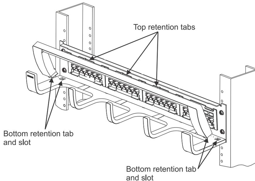
2. Position front bezel at an angle as shown and insert two bottom retention tabs into slots in cord management.
