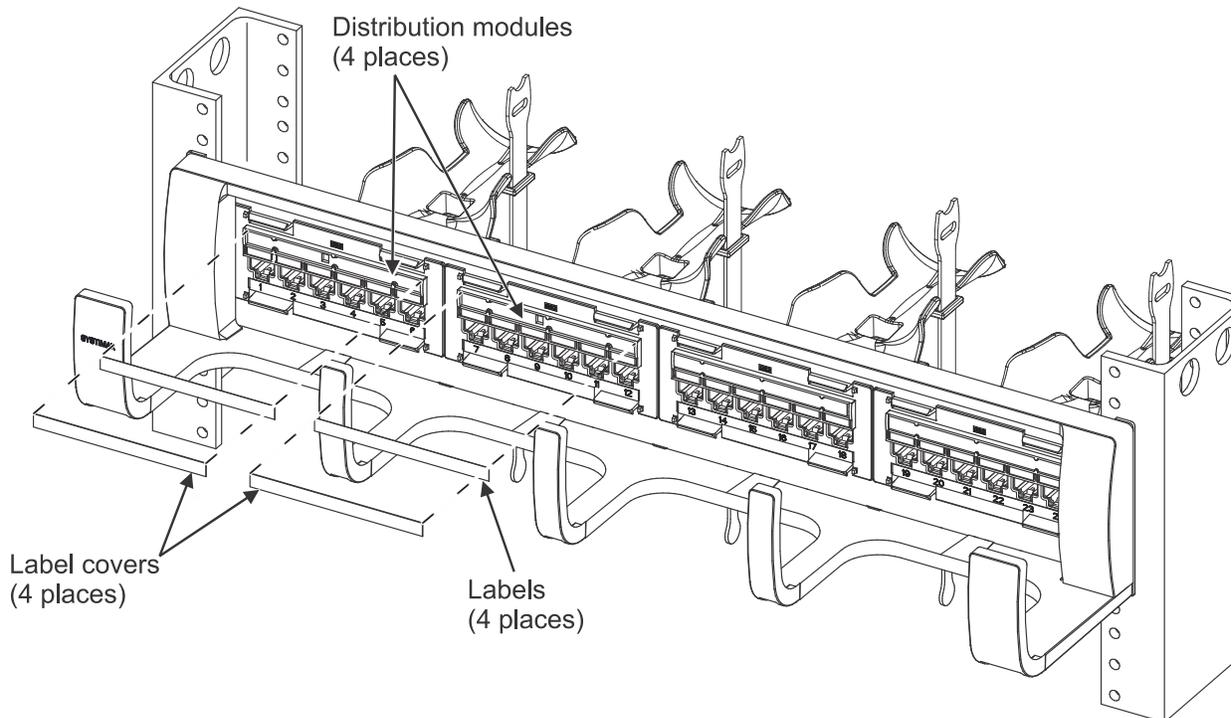
4. Print the port designations on the white label cards provided. Slide labels and label covers into the label holders from either end. Each label holder will accommodate labels up to .265 inches (6.7mm) high x 3.50 inches (89mm) wide.
