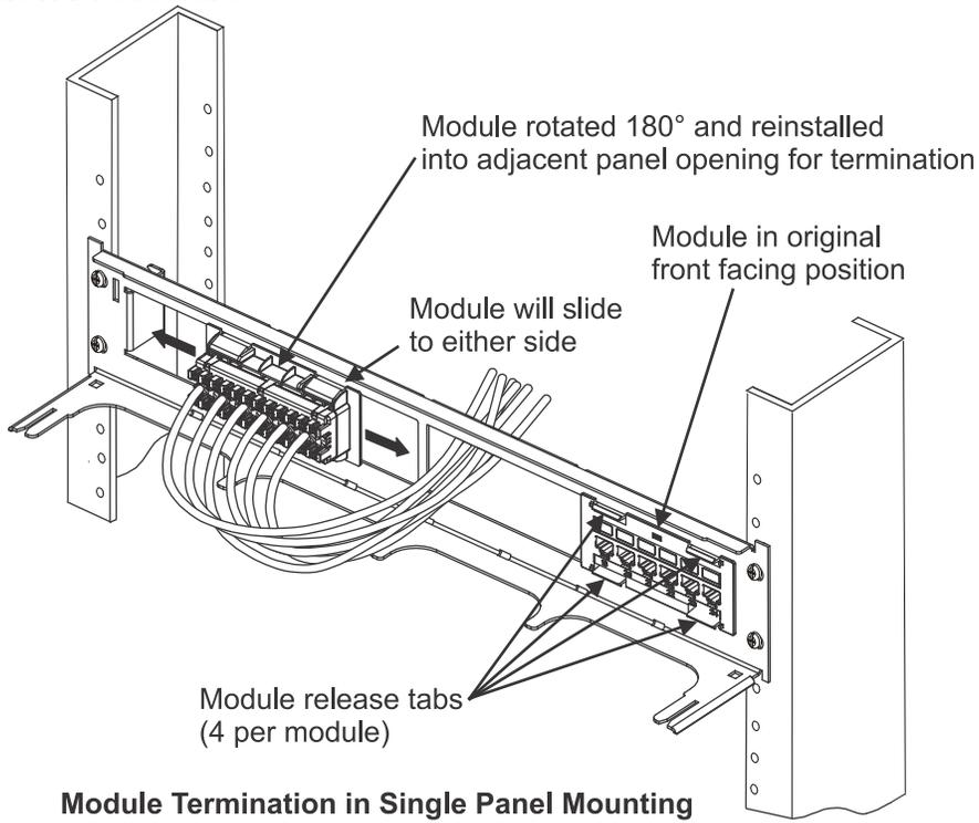
**Module Termination in Single Panel Mounting**
