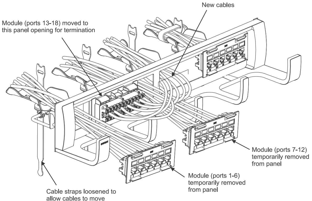
1. Remove two terminated or un-terminated modules (ports 1-6 and ports 7-12) from panel opening to free up space for new termination sequence. Leave modules out of panel.
