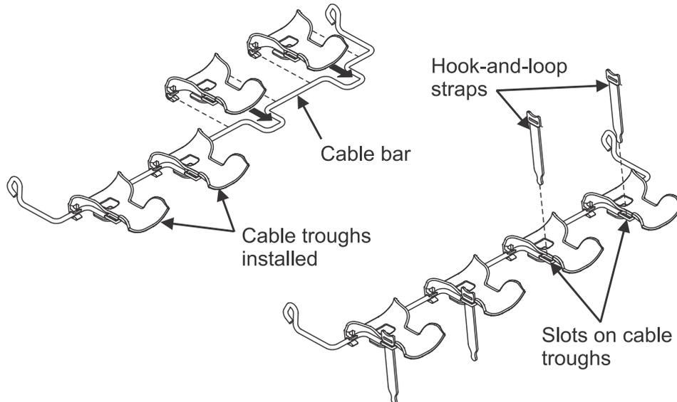
1. Attach the four cable troughs onto bar as shown and insert four hook-and-loop straps into slots in cable troughs.
