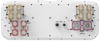
20-port sector antenna, 4x 617-894, 8x 1695-2690 MHz 65° HPBW and 8x 2300-4200 MHz, Beamformer, 7x RET
