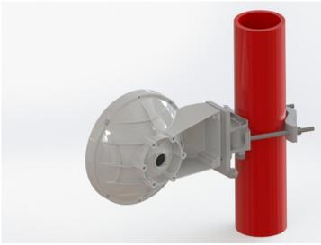
0.2 m | 0.67 ft ValuLine® High Performance Low Profile Antenna, dual-polarized, 71.000–86.000 GHz, custom flange and color, polymer radome without flash, standard pack—one-piece reflector
