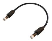
HELIAX  $\ensuremath{\mathbb{R}}$  1/2" Superflexible SureFlex  $\ensuremath{\mathbb{R}}$  Jumper with interface types 4.3-10 Male and N Male with HELIAX  $\ensuremath{\mathbb{R}}$  SureGuard weatherproofing, 3m
