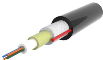
Fiber indoor/outdoor cable, Gel-filled loose tube, 4 fiber, Singlemode G.657.A1, Meters jacket marking, Black jacket color, Dca flame rating
