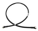
HELIAX® 1/2" SureFlex® Jumper with interface types 4.3-10 Male and 4.3-10 Male, 1m, with black non-halogenated fire retardant polyolefin jacket
