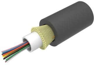
Indoor/Outdoor Low Smoke Zero Halogen, LazrSPEED® Central Loose Tube Fiber Optic Cable, 12-fiber, Multimode OM4, Gel-filled, black. Provides Rodent Resistance.
