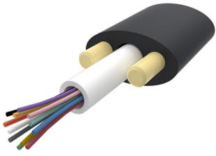
Fiber outdoor drop cable, LightScope® ZWP Self-Supporting All-Dielectric, Singlemode G.652.D and G.657.A1, 24 fiber, Arid Core construction, Gel-filled, central loose tube, no ripcords, Feet jacket marking, Black jacket color, 2000 ft
