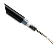
Fiber Optic Outside Plant Cable, 24-core, ECSS (Electro Chrome Coated Steel) Armored, Loose-tube, Gel-filled, 9/125 µm, OS2, Singlemode, Black cable jacket
