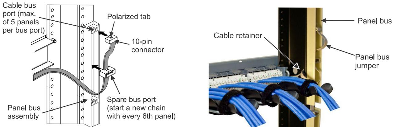
1. Unfold panel bus jumper and insert female 10-pin connector into the nearest cable bus port on panel bus assembly.
