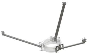
Kicker Support Arms, 3" x 3" x 96" Angle with Connecting Brackets and Hardware for 3" to 6" square or 3-1/2" to 4-1/2" OD Stand-offs, 3 sectors. Attaches to MUK-PLK7 collar - not included.
