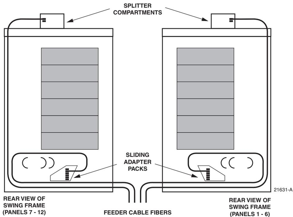
**Figure 15. Feeder Cable Typical Configuration**
