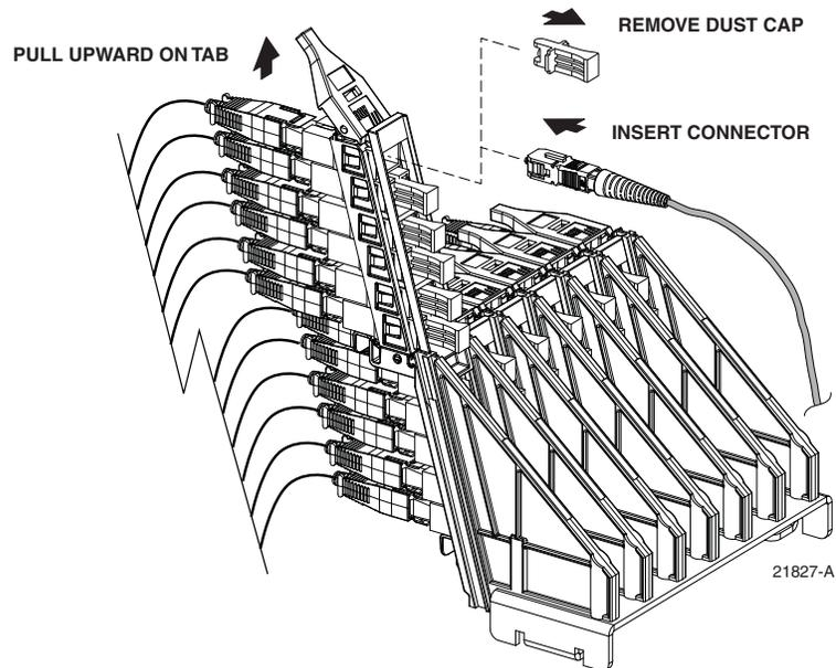
**Figure 35. Adapter Pack Raised to Access Position**
