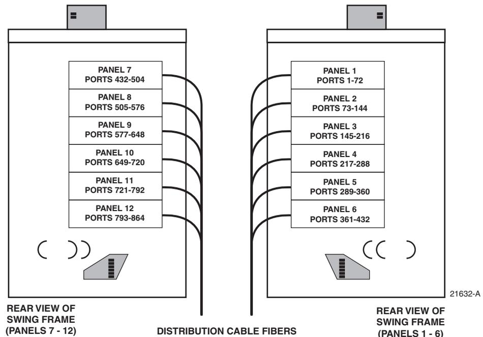
Figure 16. Distribution Cable Configuration
