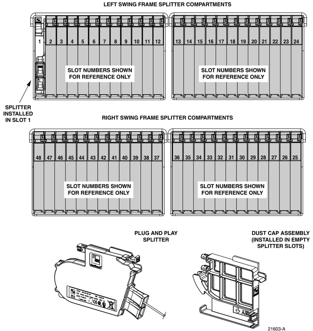
**Figure 18. Splitter Compartment Mounting Slot Assignments**
