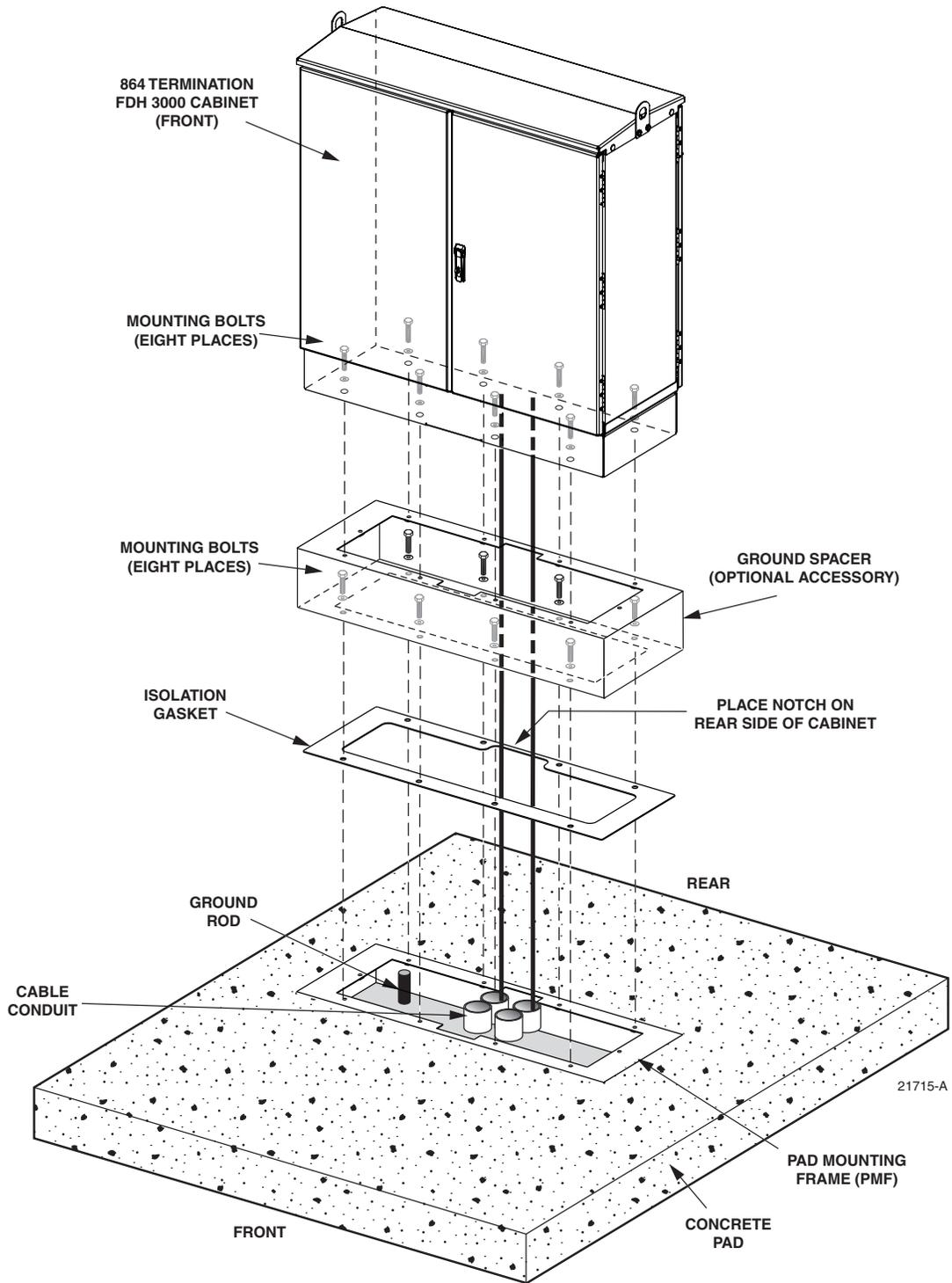
**Figure 12. Mounting the 864 Termination FDH 3000 Pedestal-Mount Cabinet on the Concrete Pad**
