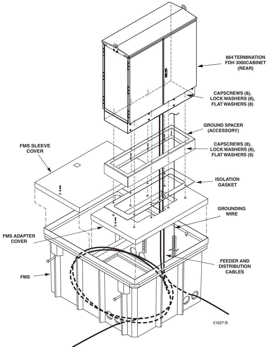
Figure 5. Mounting the 864 Termination FDH 3000 Pedestal-Mount Cabinet on the FMS
