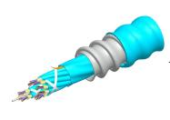
Fiber indoor cable, LazrSPEED® Riser/LSZH rated, MPO Trunk, interlocking aluminum armored, Multimode OM4, 64 fiber, Gel-free, Feet jacket marking, Aqua jacket color, B2ca flame rating
