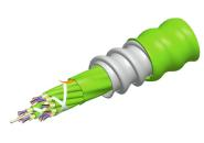
Fiber indoor cable, Riser/LSZH rated, MPO Trunk, interlocking aluminum armored, Multimode OM5, 96 fiber multi-unit with 8 fiber subunits, Gelfree, Feet jacket marking, Lime green jacket color, B2ca flame rating
