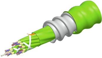
Fiber indoor cable, Riser/LSZH rated, MPO Trunk, interlocking aluminum armored, Multimode OM5, 144 fiber multi-unit with 8 fiber subunits, Gel-free, Feet jacket marking, Lime green jacket color, B2ca flame rating
