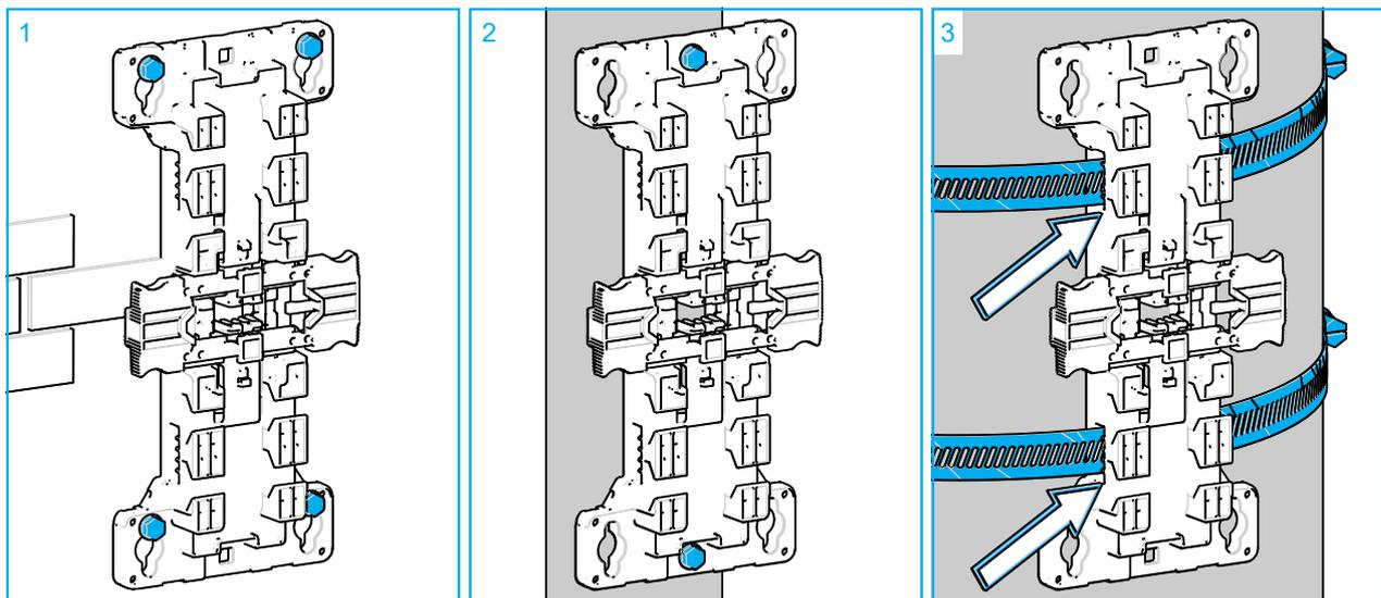
1 Mount the UMB on a flat surface with 4 screws.
