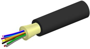
Fiber indoor/Outdoor cable, OFNR/LSZH Riser Rollable Ribbon Dual Rated Backbone, 48 fiber, Singlemode G.657.A2/B2, Feet jacket marking, Black jacket color, Cca flame rating
