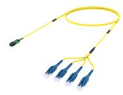
Singlemode MPO8 APC non-pinned to LC/UPC Uniboot Ruggedized fanout Cable, 8-Fiber, Dual Rated (OFNR/LSZH), 8 fiber PmP 2.0 mm
