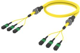
Singlemode MPO12 APC (pinned) to MPO12 APC (pinned) Fiber Trunk Cable Assembly, 36-Fiber, Armored Indoor Dual Rated (OFNR/LSZH)
