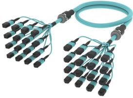
Ultra Low Loss (ULL) OM4 MPO12 UPC (pinned) to MPO12 UPC (pinned) Fiber Trunk Cable Assembly, 192-Fiber, Armored Indoor Low Smoke Zero Halogen (LSZH)
