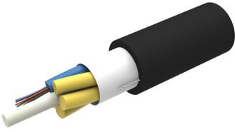
Fiber Indoor/outdoor Cable, Low Smoke Zero Halogen / 12 fiber Microsheath, Gel-free , Meters jacket marking, Black jacket color, B2ca flame rating
