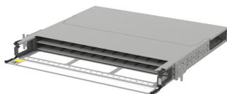
Propel 1RU fixed tray fiber panel, accepts Propel components, providing up to 48 duplex LC ports, 48 MPO ports or 96 SN ports (192f)
