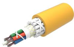
TeraSPEED® Single Jacket/Single GRP Armor, Gel, Indoor/Outdoor Stranded Loose Tube cable. Provides Rodent Resistance. Tube Colours Red, Blue, 10 x Green
