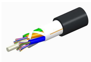
Fiber indoor/outdoor cable, TeraSPEED®, Single Jacket All-Dielectric, Low Smoke Zero Halogen (LSZH), 48 fiber, Multimode/Singlemode, Gel-Free, Stranded Loose Tube, Black jacket color, Feet cable marking, Eca flame rating
