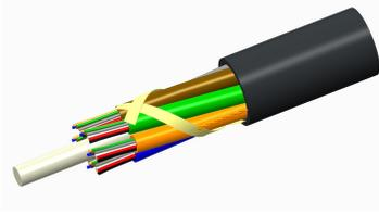
Fiber OSP cable, LightScope® ZWP Blown Micro Single Jacket, 96 fiber, All-Dielectric Stranded Loose Tube Arid-Core™ Construction, Gel-filled, Singlemode G.652.D and G.657.A1, Meters jacket marking, Black jacket color
