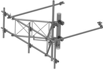
G23RHDXL PIM OPTIMIZED SPACING High Capacity Sector Frame with extended 10' Spine for RRU Mounting & extended frame for sites requiring increased sector to sector antenna spacing. 2 7/8in OD x 11ft face with (3) 2-7/8in OD x 126in Antenna pipes
