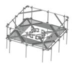
Four-sector HD Platform for 10" to 30" Monopoles, 12ft x 3.5" OD Face pipes, 2.88" OD Top Rail, includes (12) 2.88" OD x 96" antenna pipes
