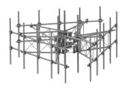
G23RHDXL PIM OPTIMIZED SPACING High Capacity Monopole platform with extended 10' Spine for RRU Mounting & extended frame for sites requiring increased sector to sector antenna spacing. 2 7/8in OD x 15ft face with (15) 2-7/8in OD x 126in Antenna pipes
