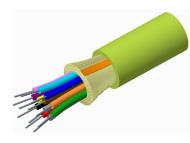
Fiber indoor cable, Low Smoke Zero Halogen Distribution, 2 fiber single-unit, Multimode OM5, Meters jacket marking, Lime green jacket color
