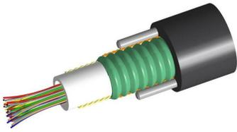
Fiber OSP cable, TeraSPEED® Single Jacket/Single Armor, Gel-Filled, 8 fibers, Outdoor Central Tube, Singlemode G.652.D and G.657.A1, Feet jacket marking, Black jacket color
