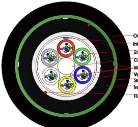
Outer Jacket PE /2mm Inlay Measuring Tape 2mm Stranded Gel Loose Tube / 12F Central Strength Member Water Blocking Tape/Yarns Water Blocking E-Glass Yarn Steel armoure Tape Inner PE Jacket / 1.7mm Ripcord
