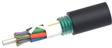
Fiber OSP cable, LightScope® ZWP Single Jacket/Single Armor, Gel-Free, 48 fibers, Stranded Loose Tube, Singlemode G.652.D and G.657.A1, Feet jacket marking, Black jacket color
