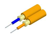
Fiber indoor cable, 1.6 mm diameter, Plenum rated, Zipcord 2-fiber, Singlemode G.657.A2, Feet jacket marking, Orange jacket color
