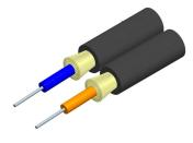
Fiber indoor cable, 1.6 mm diameter, Plenum rated, Zipcord 2-fiber, Singlemode G.657.A2, Feet jacket marking, Black jacket color
